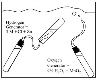
"Pre-form" tube being filled with approximately 2/3rds H<sub>2</sub>:1/3rd O<sub>2</sub> by water displacement
